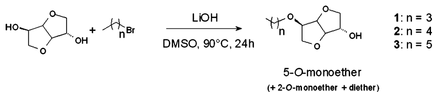
Scheme 1 Synthesis of 5- O -monobutyl isosorbide 1, 5- O -monopentyl isosorbide 2 and 5- O -monohexyl isosorbide 3.
